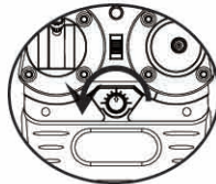
Counterclockwise rotation vernier adjustment knob
